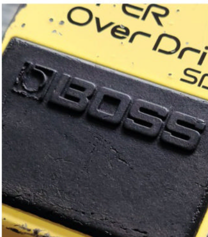
The SD-1 was a refinement of the circuit in the original OD-1 OverDrive, with more gain and the addition of a tone knob.
